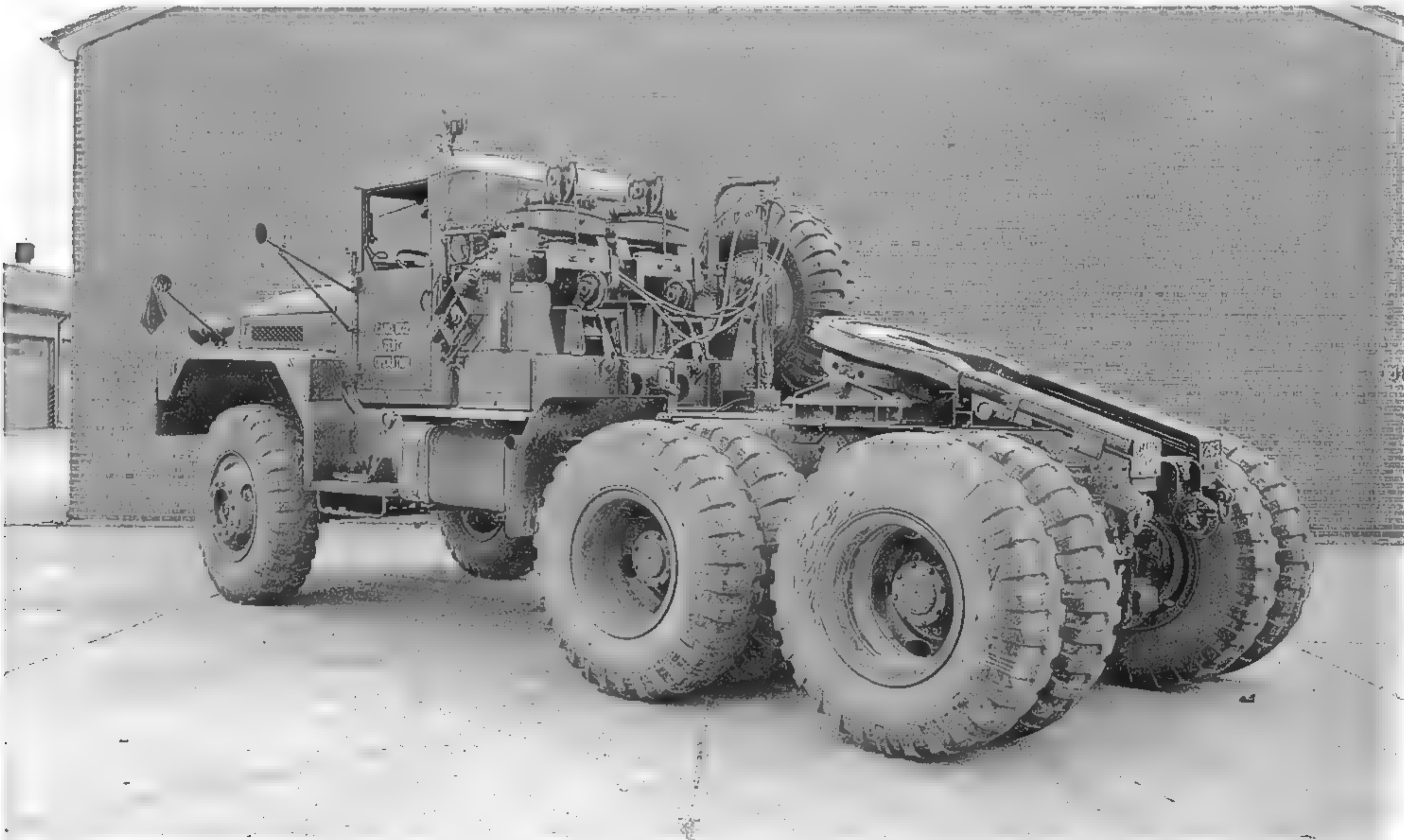
The M123 had dual rear winches. The two winches were operated in tandem, with their ropes crossed, to guide disabled tanks onto the trailer towed by the tractor. The rear winches were equipped with level-wind devices and cable tensioners. The siren on the left front fender was a popular non-standard item. (Photo courtesy of the Patton Museum, Fort Knox, Kentucky)
